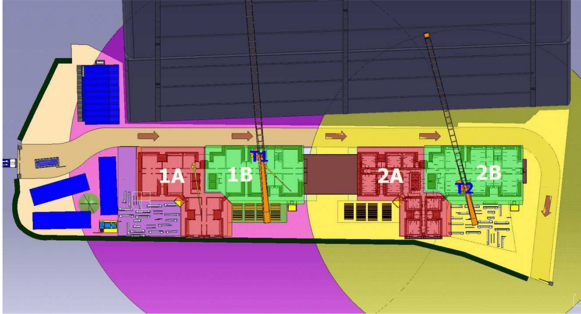
Fig. 5. The location of the two tower crane and the four bays
