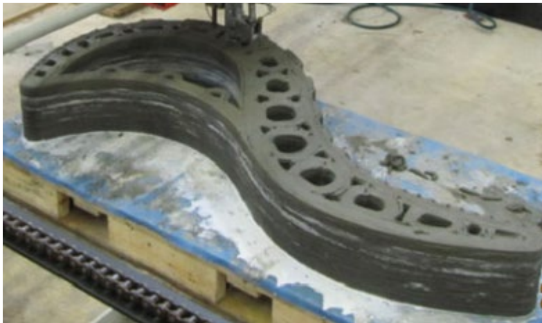
4 5 Figure 2 - A concrete printed object: Note the ribbing on the side from the layered approach (Source: Austin, Lim & Le, 6 2012)
