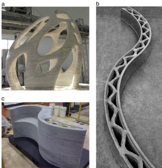
9 Figure 5 - An example of the product that each printing process can achieve (a. d-shape; a. contour crafting; c. concrete 10 printing.) (Source: Lim, 2012)
