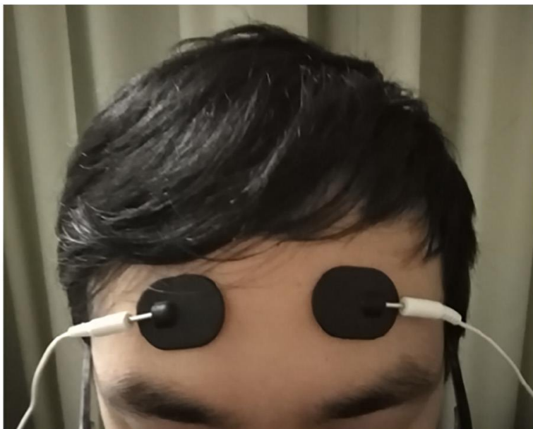
Fig. 6. Two adhesive rubber electrodes placed corresponding to the V1 branches of the trigeminal nerve ((a) schematic of the trigeminal nerve stimulation cited from Error! Reference source not found. ; and (b) a subject in the practical experiment).
