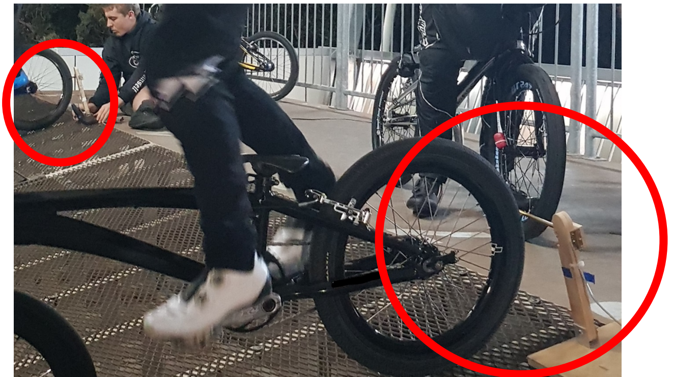
Figure 6-7 Reaction timer setup on the SX ramp.
