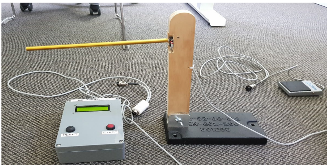
Figure 6-4 Reaction timer controller and display, ramp attachment and pedal attachment.
