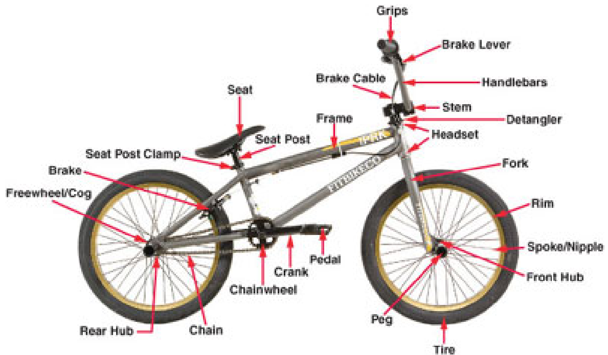
Figure 1-4. Components of a BMX bike. Reprinted from “10 Tips for Buying a Complete BMX Bike”, In BMX Transworld, Retrieved August 21 2015, From http://cdn.bmx.transworld.net/files/2009/09/1-bike-types.jpg .
