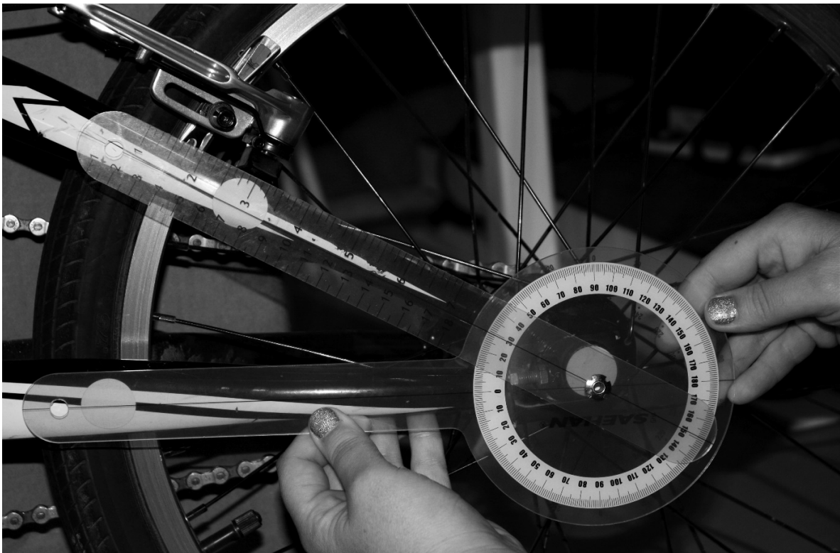
Figure 7-3 The angle between the seat stay and chain stay with the axis at the rear wheel hub was measured with a goniometer with the bike in a stable position. The stationary and movement arms of the goniometer were set so that they were aligned with the centre
