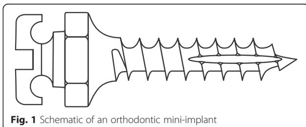
**Fig. 1** Schematic of an orthodontic mini-implant
