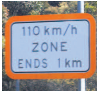
Figure 9. Sign designed to attract additional attention with fluorescent-orange border
