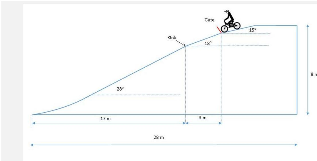
**Figure 1.** Supercross ramp design as specified by the UCI BMX Track Guidelines (Union Cycliste Internationale)
