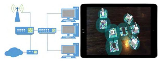
**Figure 1:** An example simple network model & the equivalent view using augmented reality markers on an iPad
