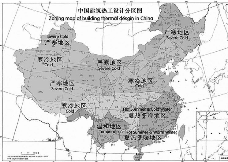
Figure 2. Zoning map of building thermal design in China (source: Thermal Design Code for Civil Building)
