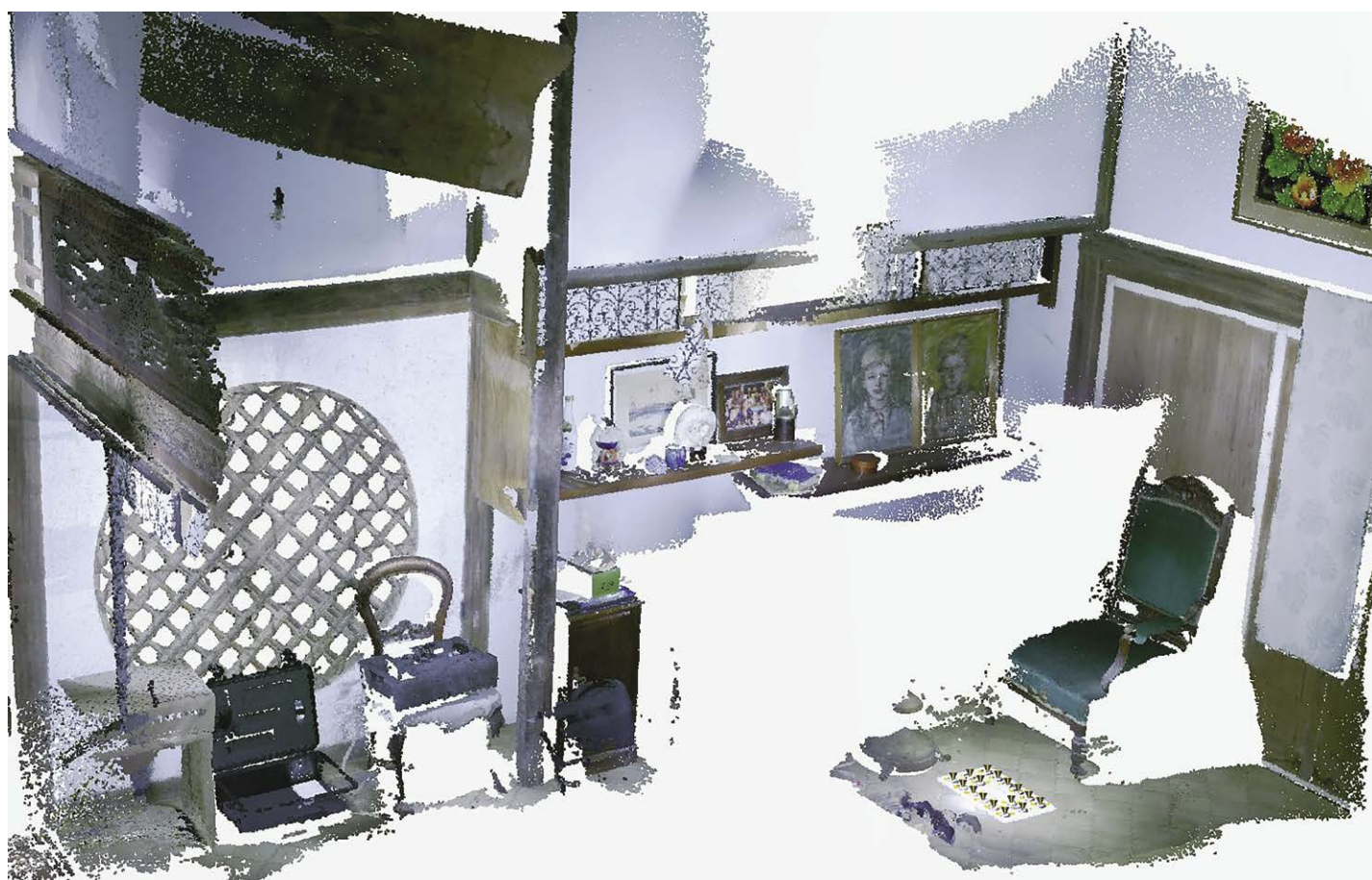
Figure 1: Raw images of small sections from the trial scan with insufficient overlap (Source: Authors, 2022)
