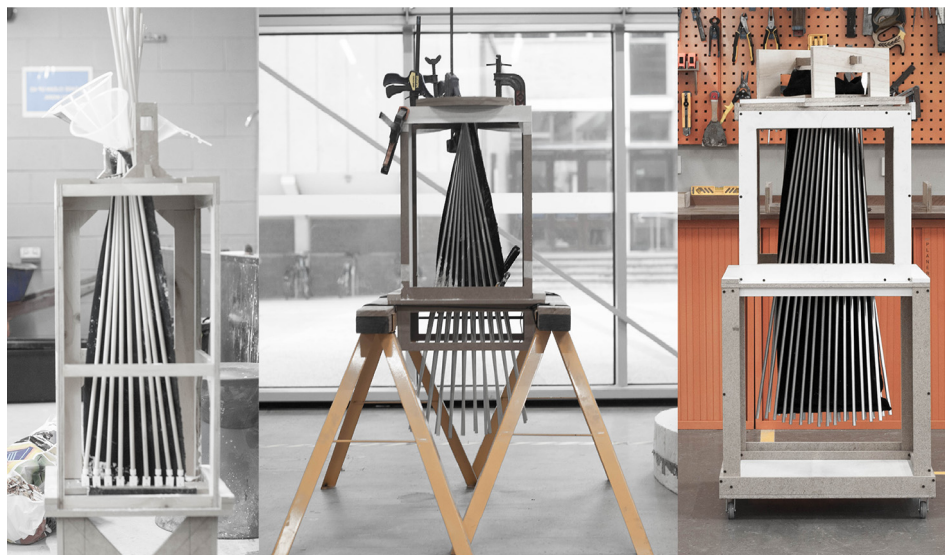
Fig. 5. Various iterations of mould design. Iterations 4 (left) and 5 (middle) are manually operated. The latest design (right) is paired with the robotic arm.
