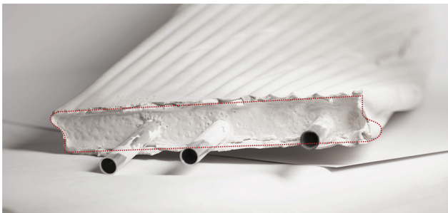
Fig. 13. Aluminium pipes embedded in the hyperbolic paraboloid panel.
