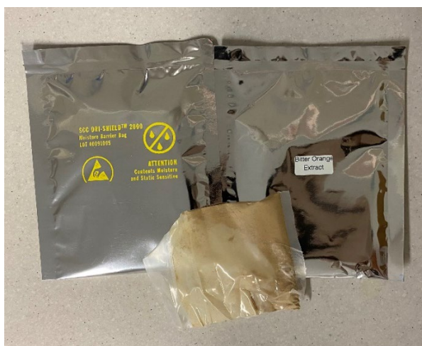
Figure 36: Photo of dry powdered bitter orange extract (SRM 3259) samples in vacuumed sealed packets
