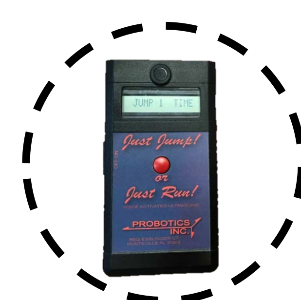
Figure 1. Just Jump System was used to capture VJ height and average ground contact time between jumps.
