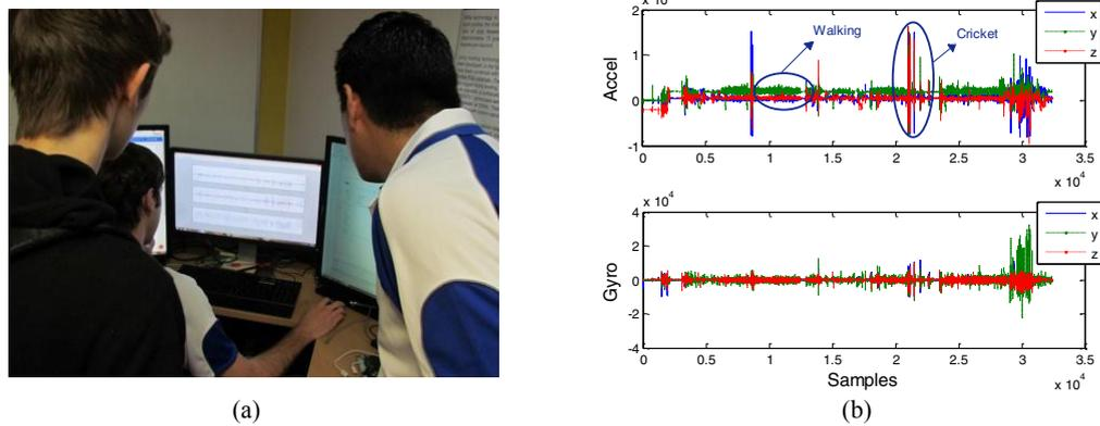
Figure 2. Students participating in Griffith University Experience day event. (A) A student receiving an interpretation on his sensor data extraction (b) data extracted from the wearable sensor (3-axis accelerometer/gyroscope) with activity classification.
