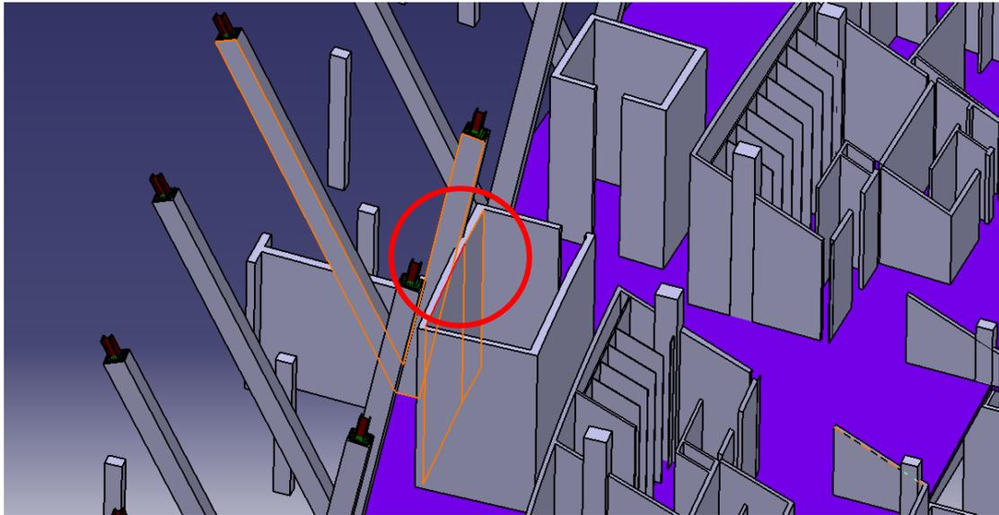
*Figure 13: A clash between a V-column and partition*
