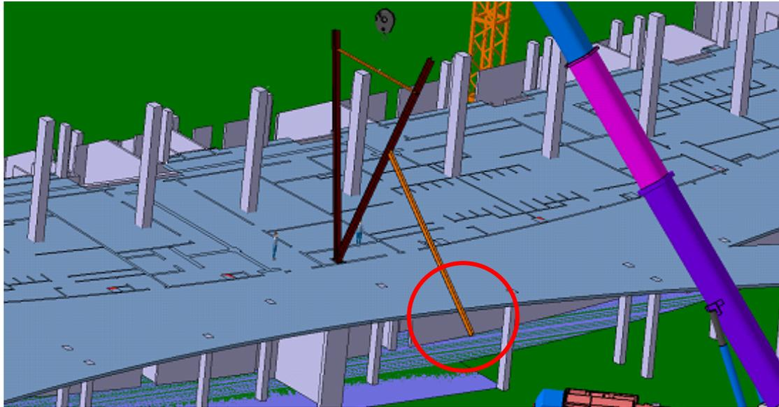
*Figure 9: The simulation of V-column installation*
