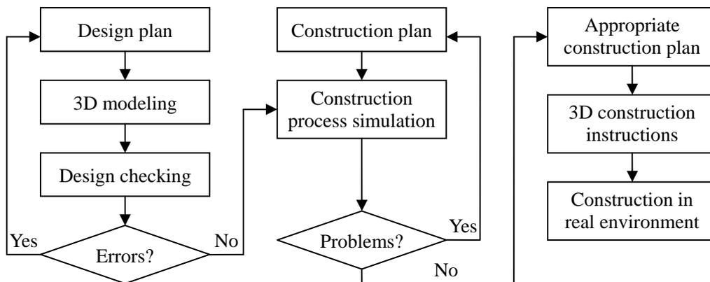
Figure 11: The flow of applying "IKEA" pattern into construction projects
