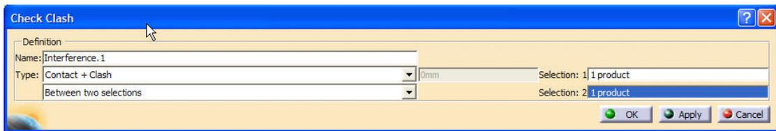
*Figure 4: Checking design errors automatically*
