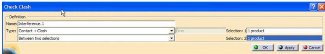
Figure 5: Automatic design error detection
