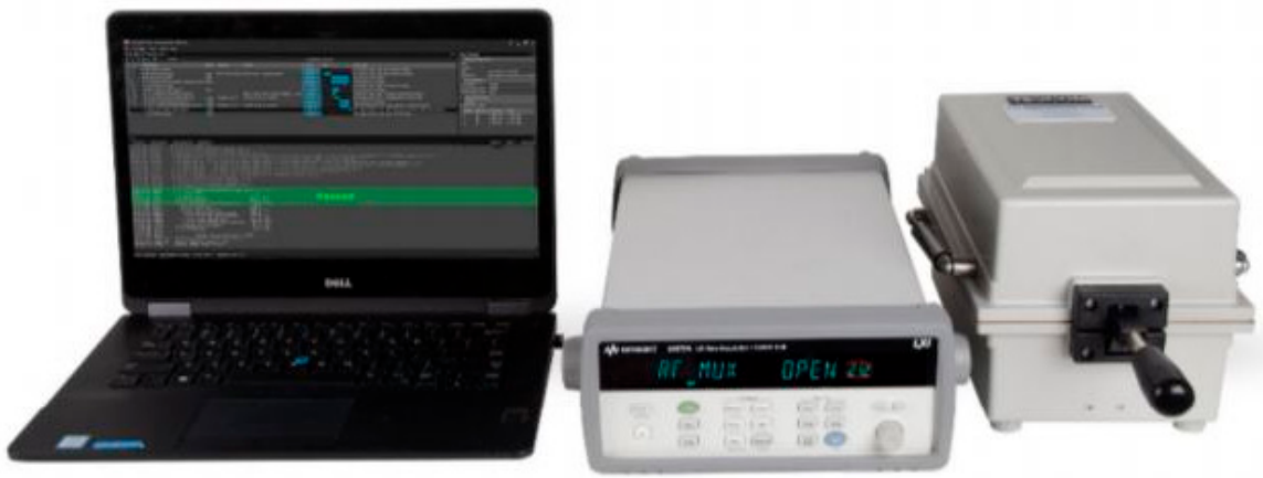
Figure 14. The test equipment for LoRa network.
