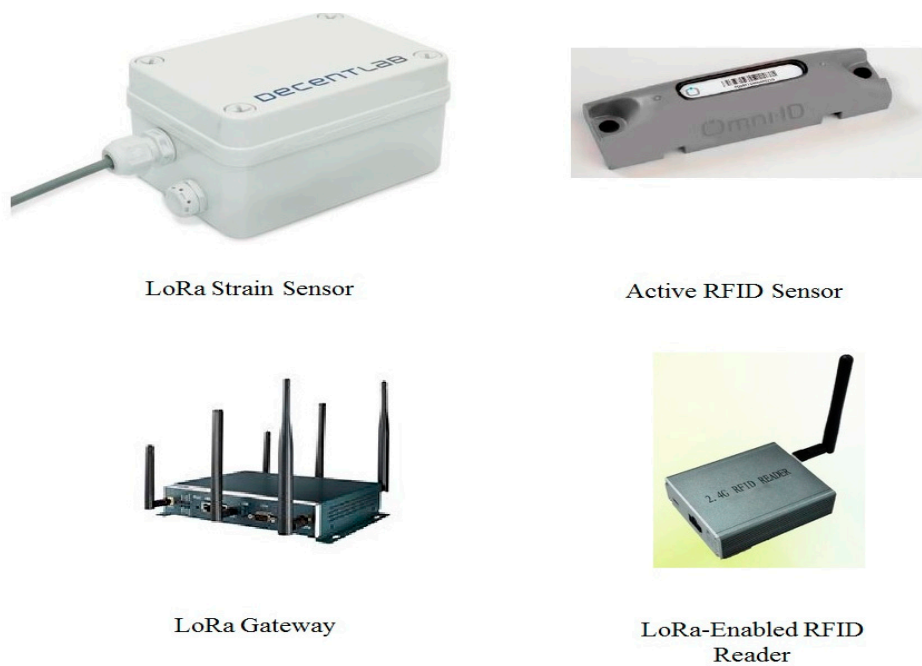
Figure 10. Pictures of the devices used in the proposed method.
