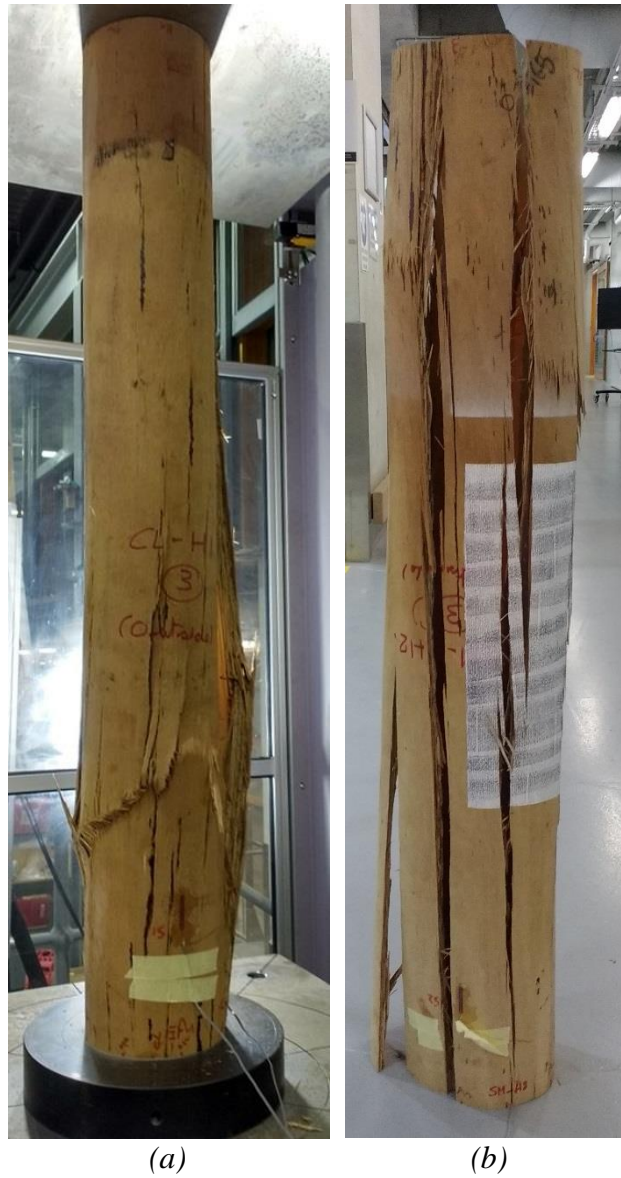
620 Figure 13: Compression tests failure modes, (a) local buckling of the wall for the compact sections 621 (shown for C_G1) and (b) sudden failure with the sections bursting into strips for the slender sec- 622 tions with no cross-banded veneers (shown for S_G2)
