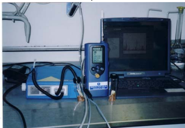
Figure 1 The E-nose and preconcentrator system in the laboratory.
