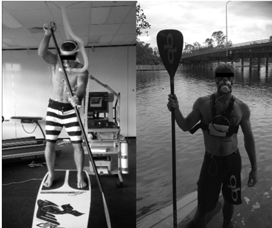
Figure 1: Lab based testing on the SUP ergometer and field based testing with the K4b2 portable unit.
