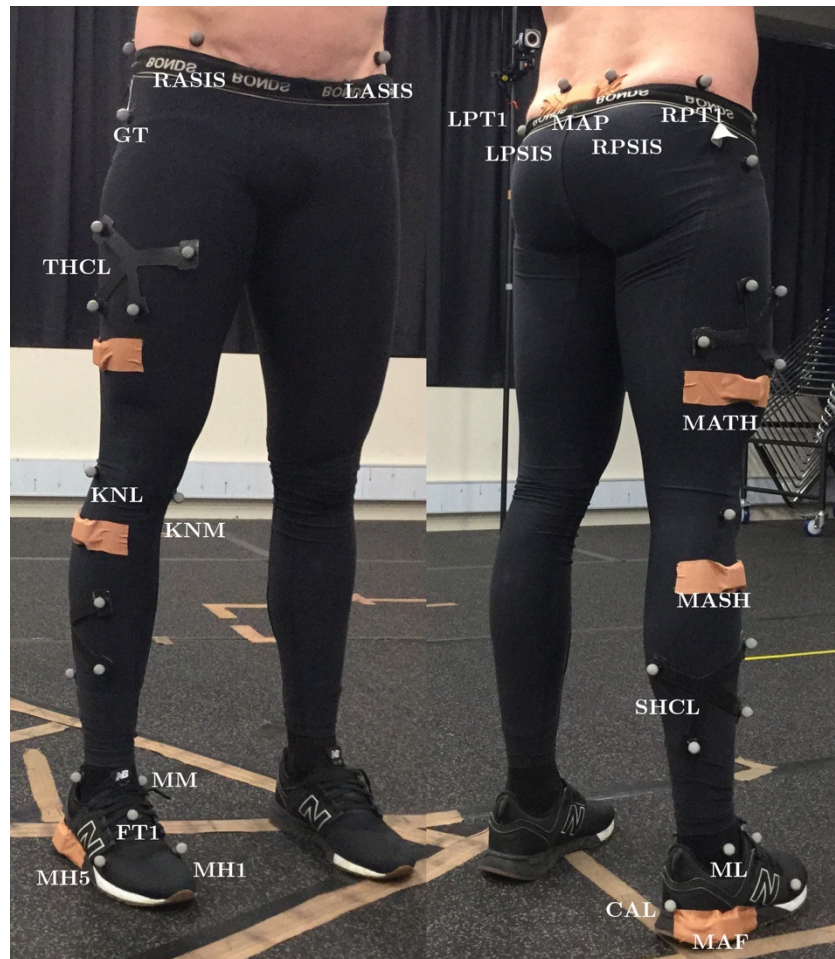
Figure 6.2 Optical motion capture (OMC) and magnetic, angular rate and gravity (MARG) sensor placement: CAL) calcaneus; FT1) foot tracking marker one; GT) greater trochanter; KNL) knee lateral; KNM) knee medial; LASIS) left anterior superior iliac spine; LPSIS) left posterior superior iliac spine; LPT1) left pelvis tracking marker one; MAF) foot MARG sensor; MAP) pelvis MARG sensor; MASH) shank MARG sensor; MATH) thigh MARG sensor; MH1) first metatarsal head; MH5) fifth metatarsal head; ML) lateral malleolus; MM) medial malleolus; RASIS) right anterior superior iliac spine; RPSIS) right posterior superior iliac spine; RPT1) right pelvis tracking marker one; SHCL) shank cluster; THCL) thigh cluster. Image reproduced with permission from respective copyright owner and person pictured.
